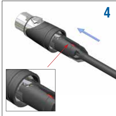
Install the cable clamp, flush to the insert making sure to align the top slot with the spring. Then push the insert & cable clamp together into the shell.
