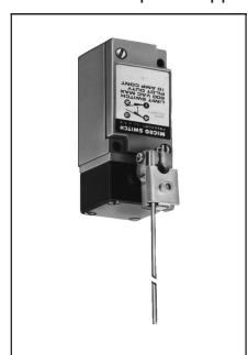
NOTE: LSS1H and LST1H switches are usually mounted with the lever down. Heavier levers, such as the LSZ54N (shown) and LSZ52D, should be used to enable gravity to help restore them to the free position. These levers are described on page A38.
