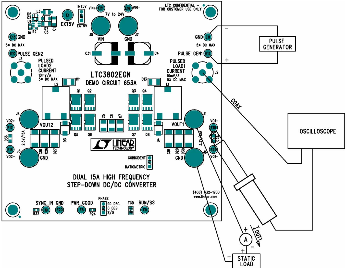
Figure 3. Equipment setup for load step testing.
