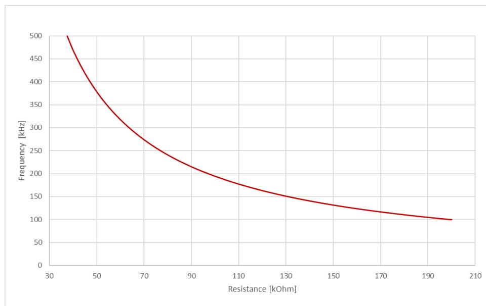
Figure 2.5. R<sub>FREQ</sub> Frequency Selector Diagram
