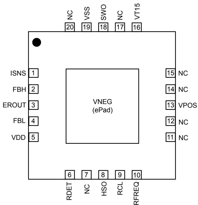
Figure 5.1. Si3404 Pinout
