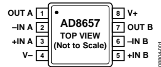
Figure 1. AD8657 Pin Configuration, 8-Lead MSOP
