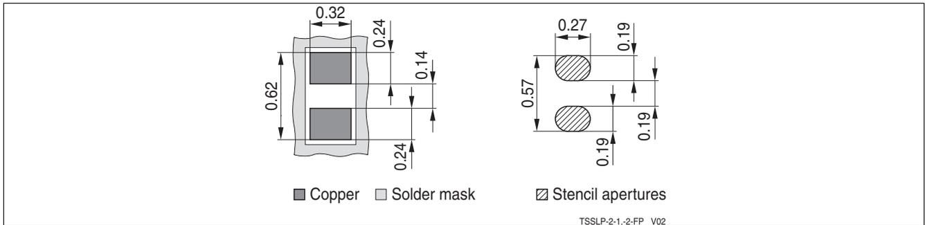
Figure 16 Package footprint for TSSLP-2-3 (dimension in mm)
