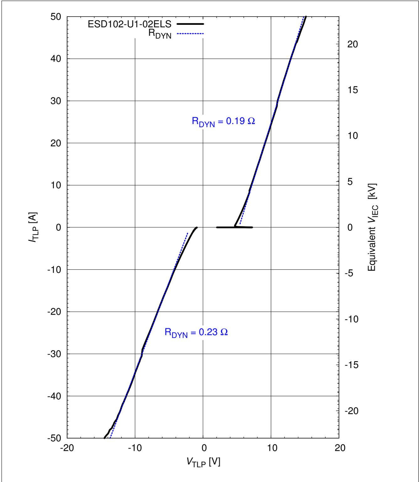
**Figure 11 Clamping voltage  $V_{TLP} = f(I_{TLP})$ , [2]**
