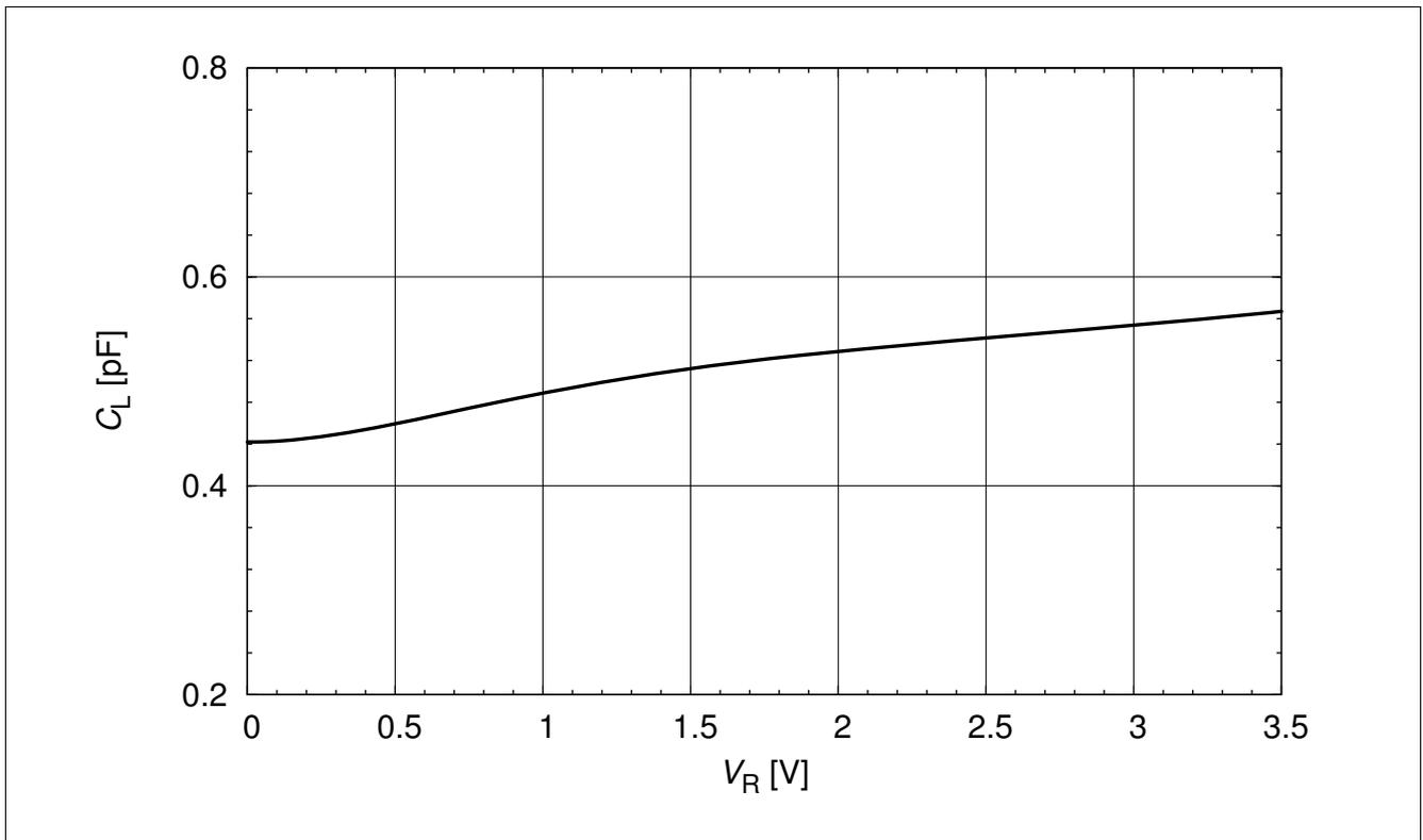
Figure 6 Line capacitance  $C_L = f(V_R)$ ,  $f = 1$  MHz, from pin 1 to pin 2
