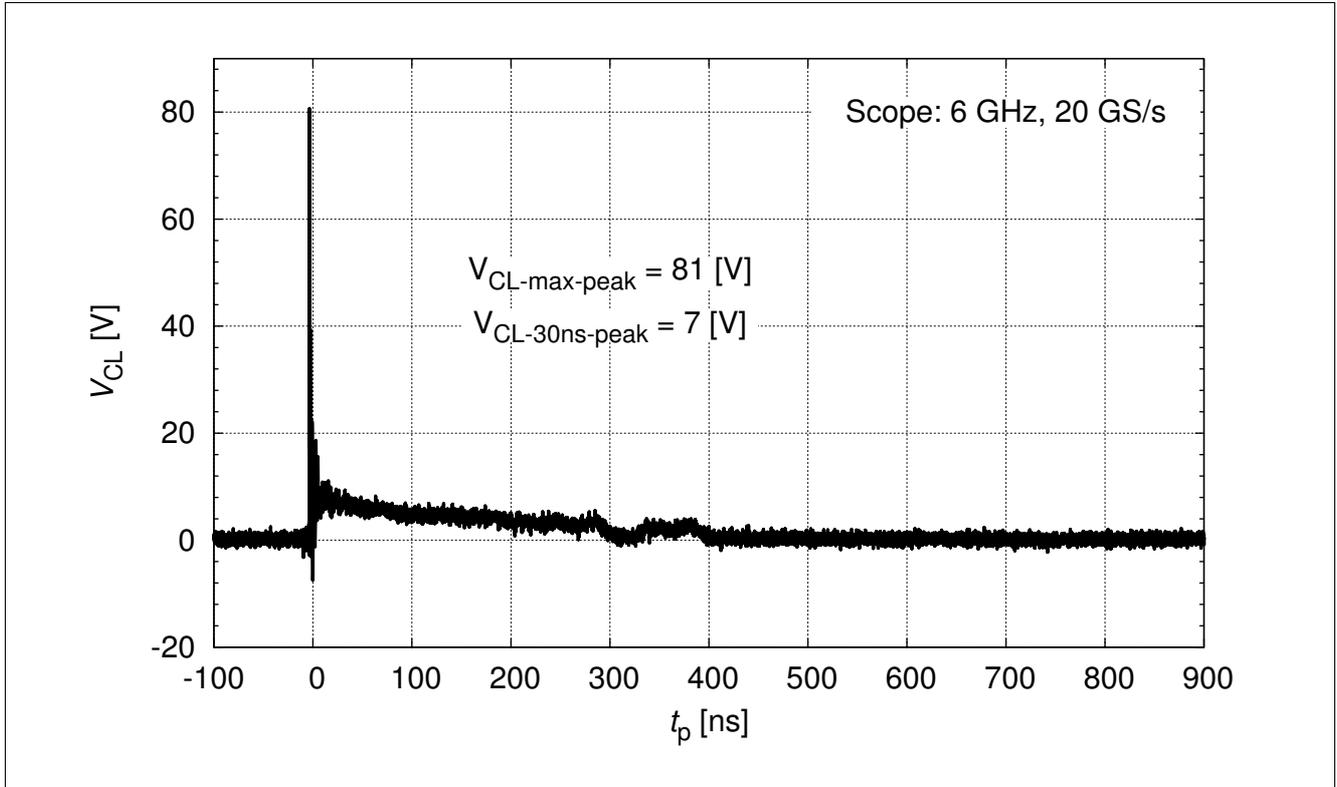
Figure 7 IEC61000-4-2  $V_{CL} = f(t)$ , 8 kV positive pulse from pin 1 to pin 2
