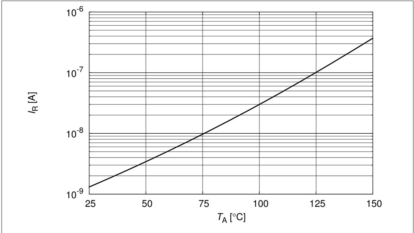
Figure 5 Reverse current  $I_R = f(T_A)$ ,  $V_R = 3.3$  V
