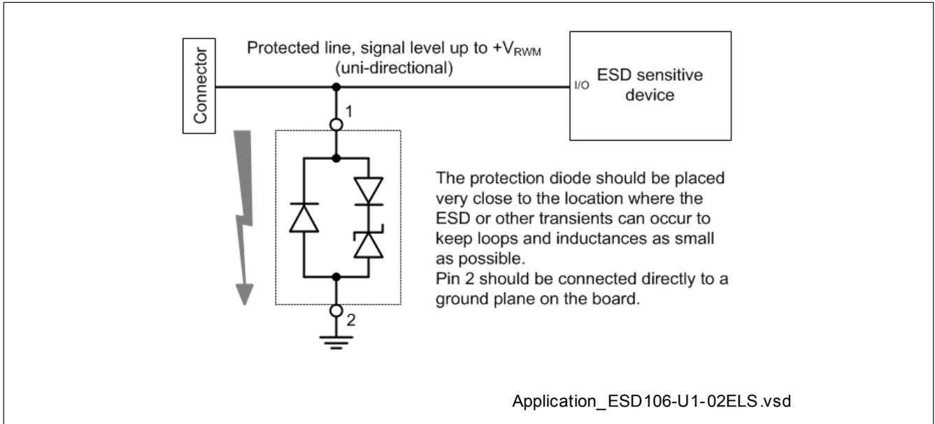
Figure 14 Single line, uni-directional ESD / Transient protection[2]
