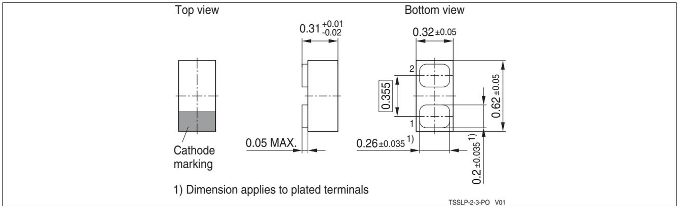
Figure 15 Package outline for TSSLP-2-3 (dimension in mm)
