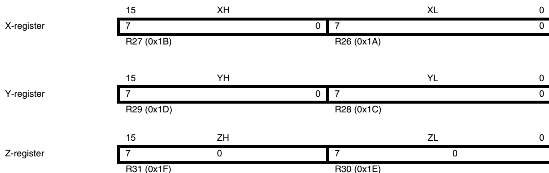
Figure 5-3. The X-, Y-, and Z-registers.
