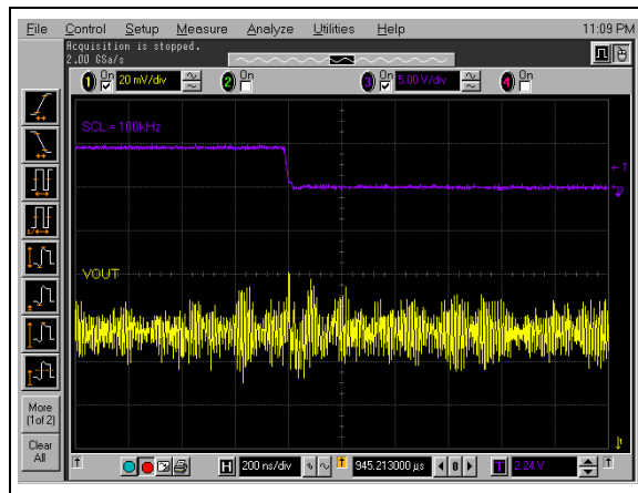
FIGURE 2-94: Digital Feedthrough (SCL signal coupling to V_{OUT} pin); V_{OUT} = 40\text{h} , F_{SCL} = 100\text{kHz} , V_{DD} = 5.0\text{V} , V_{REF} = 5.0\text{V} .
