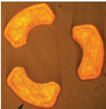
Au/Ni Barrier (Uniform plating thickness)
