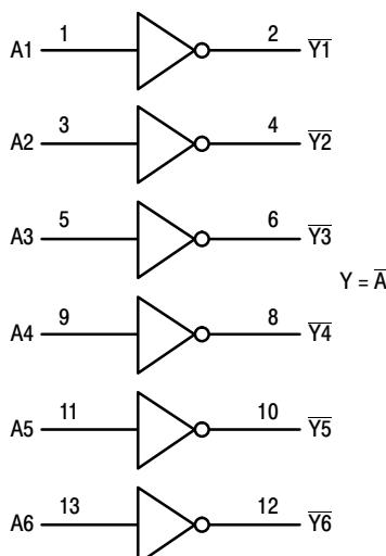
Figure 1. Logic Diagram
