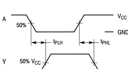
Figure 3. Switching Waveforms
