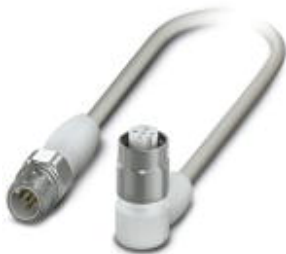
Sensor/Actuator cable, 5-position, PP-EPDM halogen-free, Gray RAL 7035, Plug straight M12, A-coded, on Socket angled M12, A-coded, Cable length: 3 m, Hygienic design, With high-grade steel knurl
