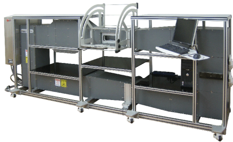
FDK Original Wind Tunnel
