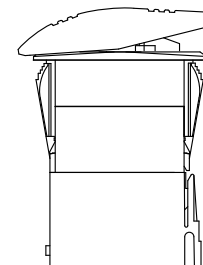
SWITCH SHOWN WITH VC1 CONNECTOR 10 TERMINAL
