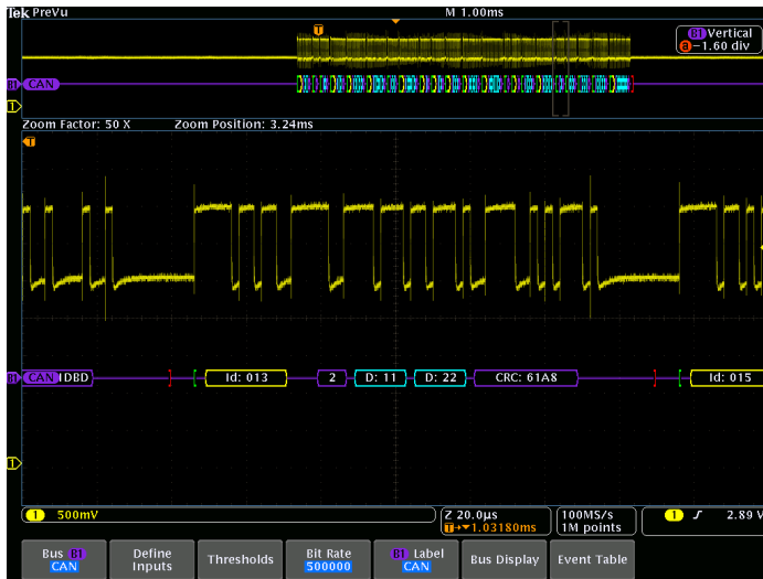
Color-coded display of a CAN bus, showing Start, DLC, Data, CRC, and Stop components of the serial signal.
