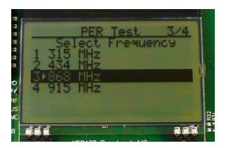
Select which frequency to use for the test. Make sure that the evaluation modules you have match the selected frequency.
