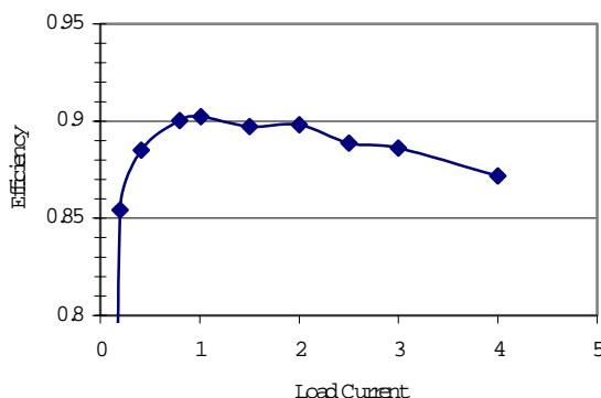
Figure 1. Efficiency, 10V  $V_{IN}$ , 5V  $V_{OUT}$
