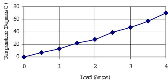
Figure 2. Die Temperature vs Output Current,  $V_{IN} = 12V$
