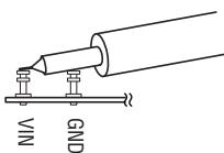
Figure 4. Scope Probe Placement for Measuring Output Ripple
