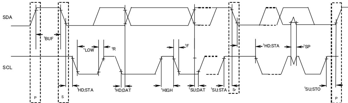
Fig. 23 Definition of timing on the I<sup>2</sup>C-bus
