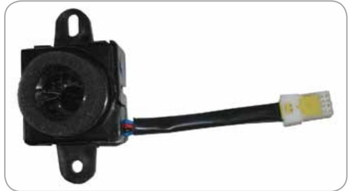
This sensor indicates temperature in the cabin of passenger cars. Since it uses a fan to continuously draw air past the thermistor for an accurate temperature reading, it requires no venturi tube.
