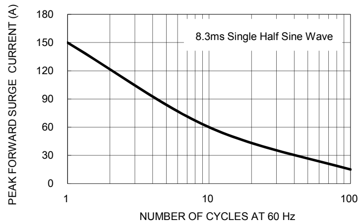
FIG. 2 MAXIMUM NON-REPETITIVE FORWARD SURGE CURRENT PER LEG
