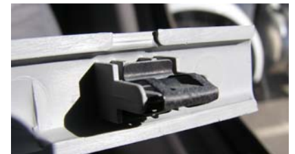
Clip to pull out slightly
