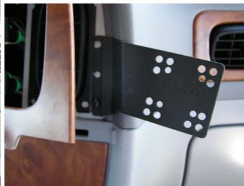
InDash fit into location with screw
