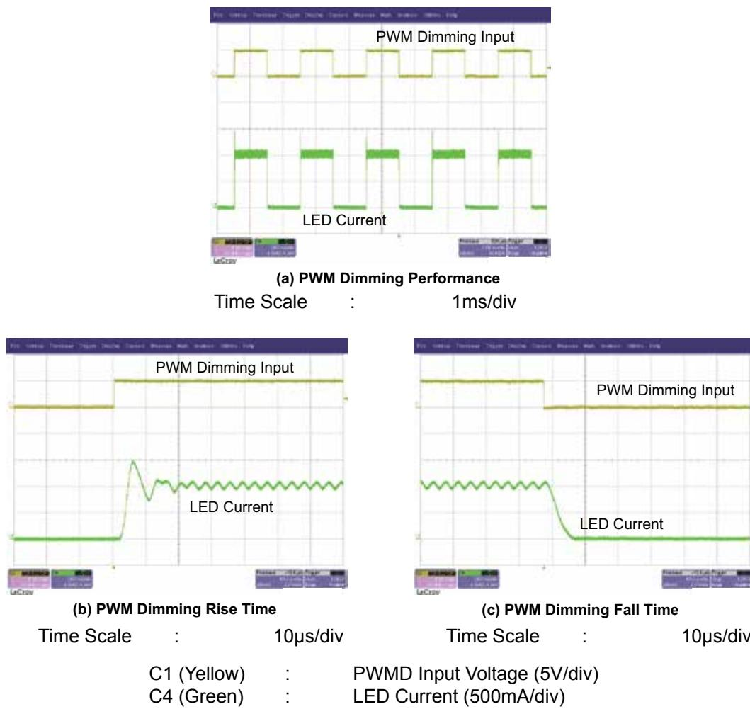
Figure 10. PWM Dimming using the ADIM pin
