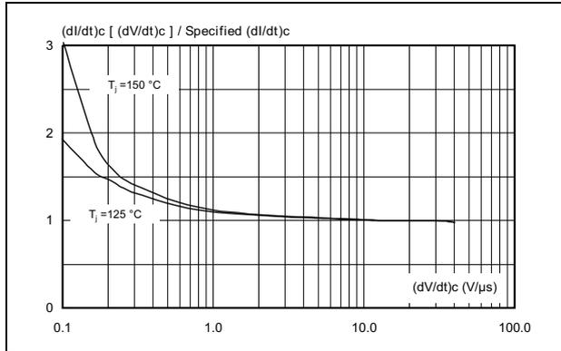
**Figure 12. Relative variation of critical rate of decrease of main current (di/dt)<sub>c</sub> versus junction temperature (typical values)**
