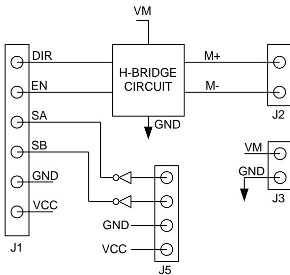
Figure 2. PmodHB3 block diagram.
