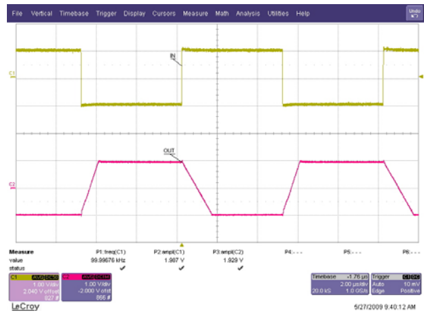
Figure 12. Inverting Large Signal Step Response
