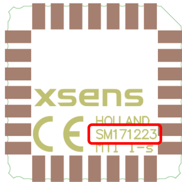
Figure 17: Location PCB number on MTi 1-series module (bottom view)
