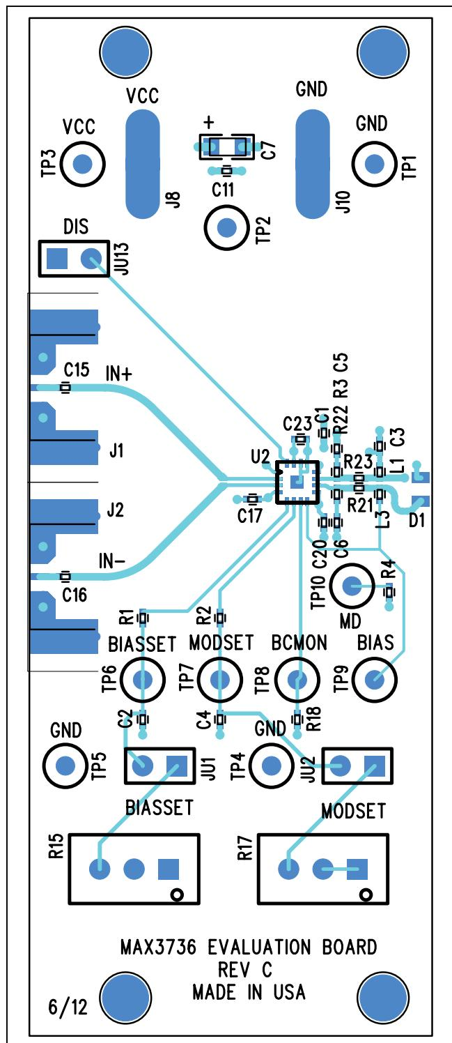
Figure 3. MAX3736 EV Kit Component Placement Guide—Component Side
