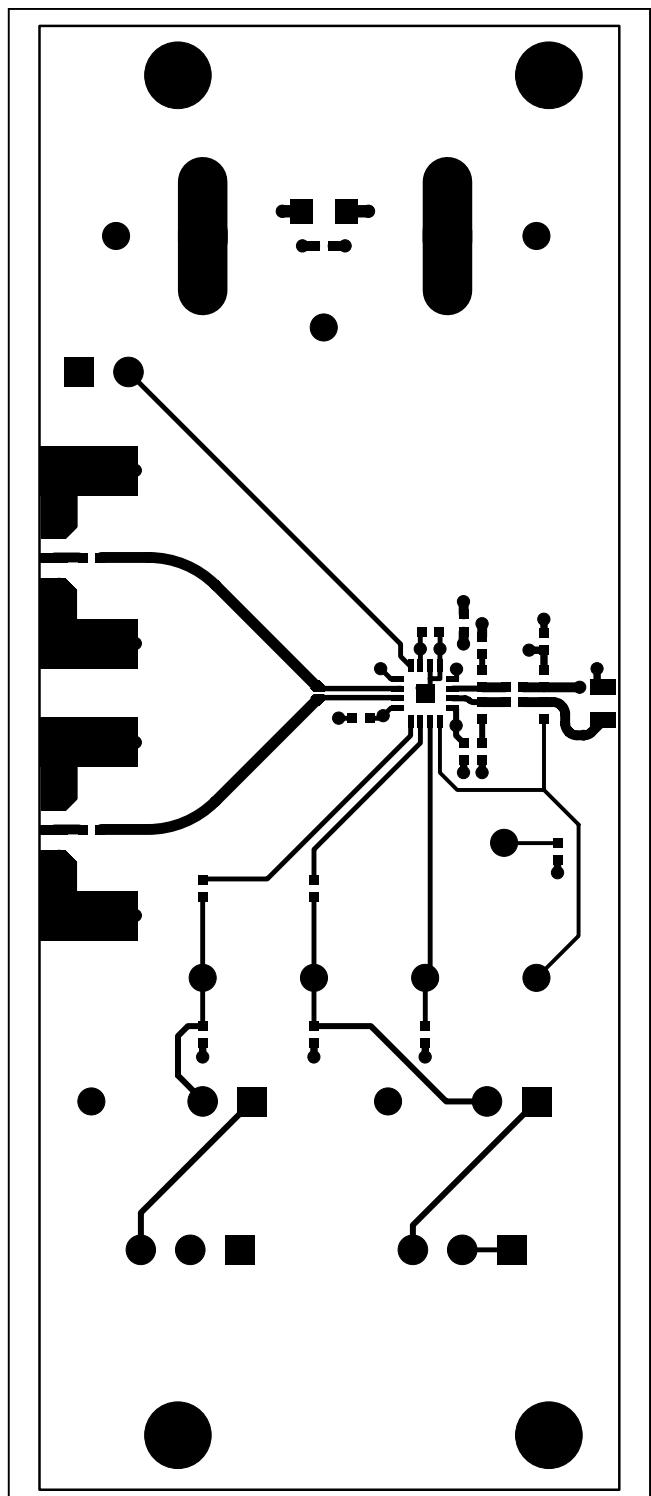
Figure 4. MAX3736 EV Kit PCB Layout—Component Side
