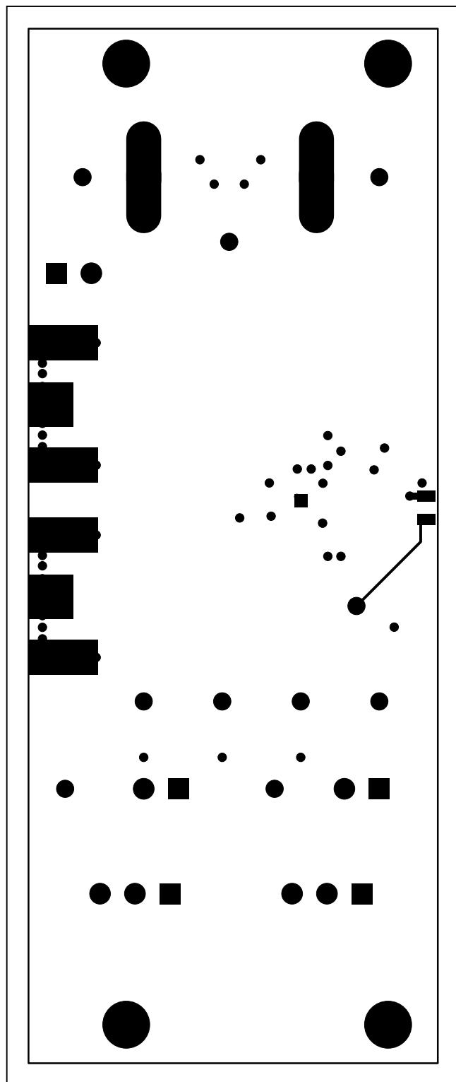
Figure 7. MAX3736 EV Kit PCB Layout—Solder Side
