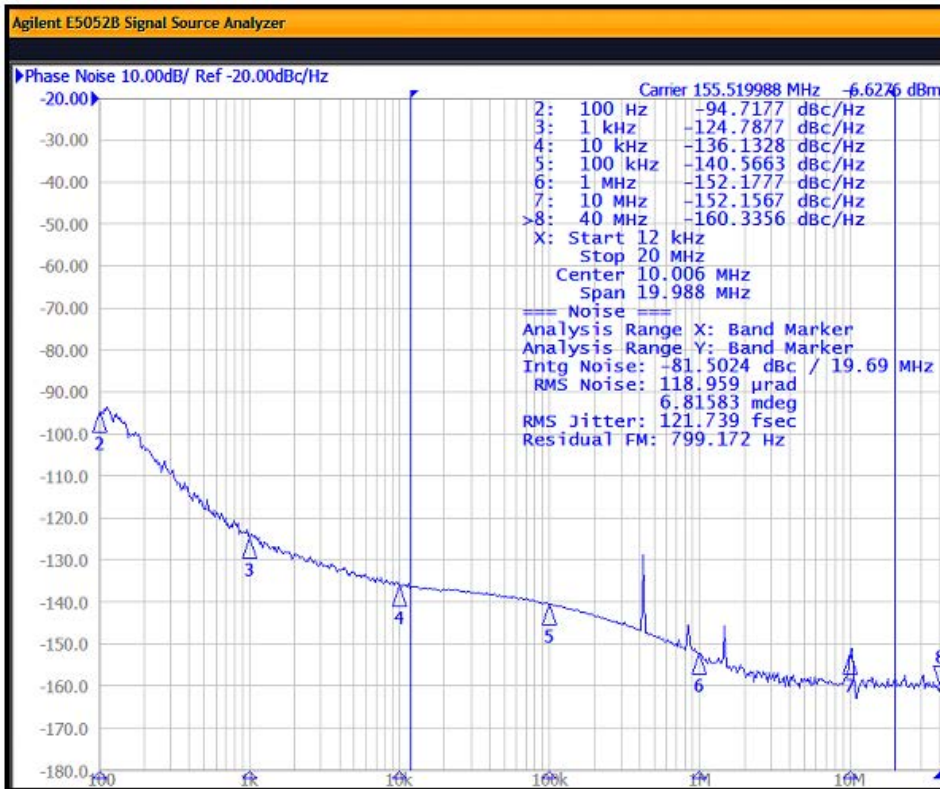
Figure 8.3. Input = 25 MHz; Output = 155.52 MHz, 2.5 V LVDS
