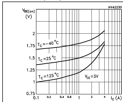
**Figure 11. Base-emitter on voltage (PNP)**
