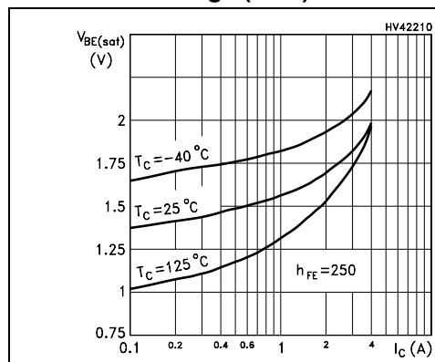
**Figure 9. Base-emitter saturation voltage (PNP)**
