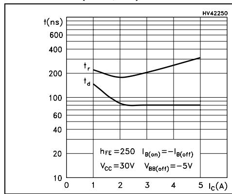
**Figure 13. Resistive load switching time (PNP, on)**
