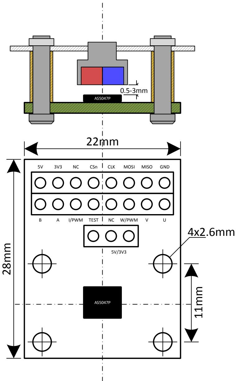
A 6x2.5mm diametric magnet must be placed over or under the AS5047P sensor, and should be centered on the middle of the package with a tolerance of 0.5mm. The airgap between the magnet surface and the package should be maintained in the range 0.5mm to 3mm. The magnet holder must not be ferromagnetic. Materials as brass, copper, aluminum, stainless steel are the best choices to make this part.
