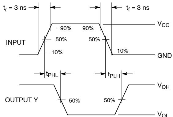
**Figure 3. Switching Waveform**
