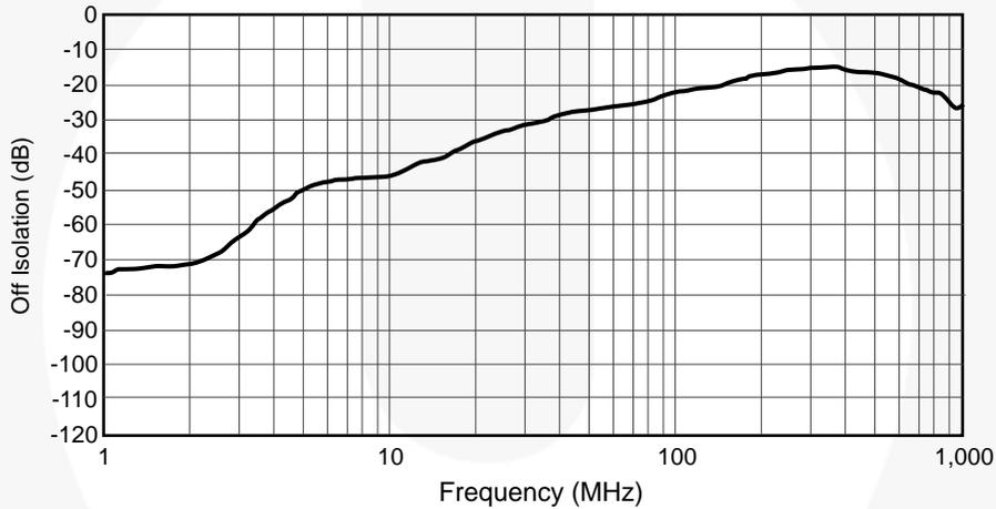
Figure 4. Crosstalk,  $V_{CC} = 2.7\text{ V to }5.5\text{ V}$
