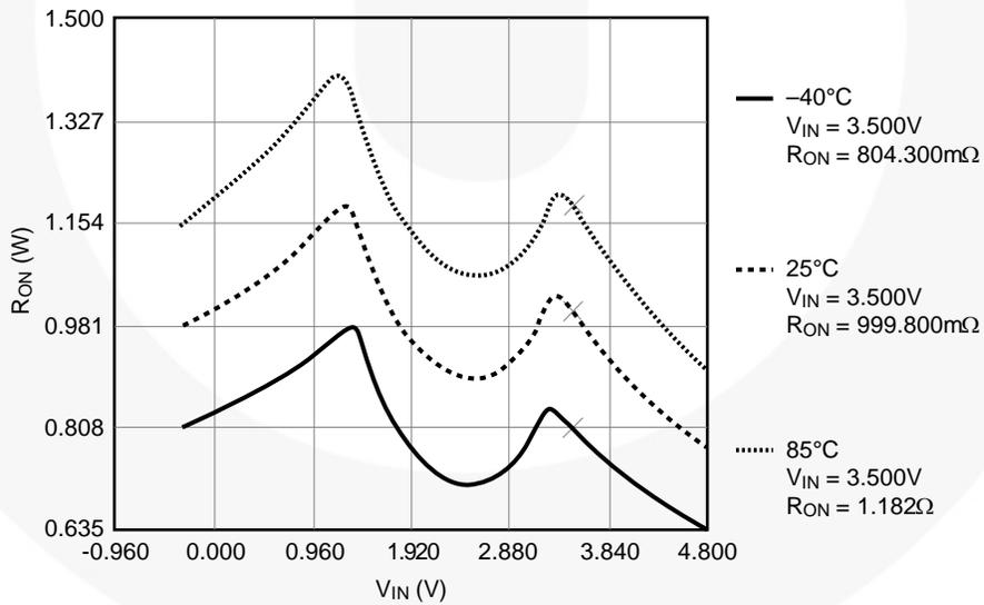
**Figure 7.** R<sub>ON</sub> Switch On Resistance, I<sub>ON</sub> = 100 mA, V<sub>CC</sub> = 4.5 V
