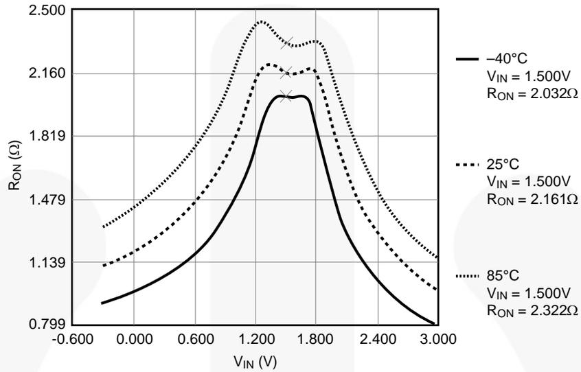
**Figure 6.** R<sub>ON</sub> Switch On Resistance, I<sub>ON</sub> = 100 mA, V<sub>CC</sub> = 2.7
