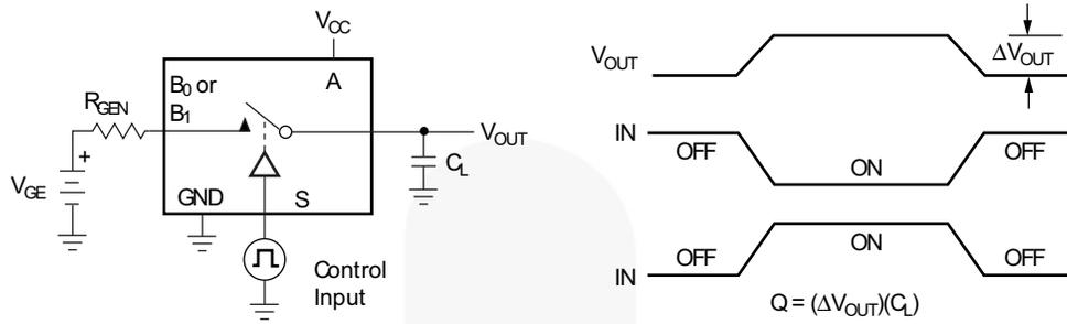
**Figure 11. Charge Injection**
