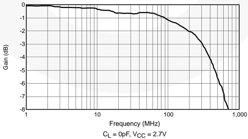
Figure 5. Bandwidth,  $V_{CC} = 2.7\text{ V to }5.5\text{ V}$
