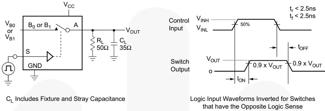
**Figure 8. Turn On / Off Timing**
