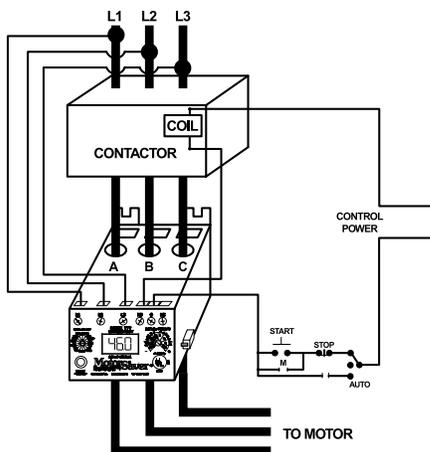
CURRENT TRANSFORMER WIRING DIAGRAM FOR MODEL 777 (80 to 800 A)
