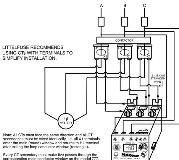
Note: All CTs must face the same direction and all CT secondaries must be wired identically, i.e. all X1 terminals enter the main (round) window and returns to H1 terminal after exiting the loop conductor window (rectangle).
