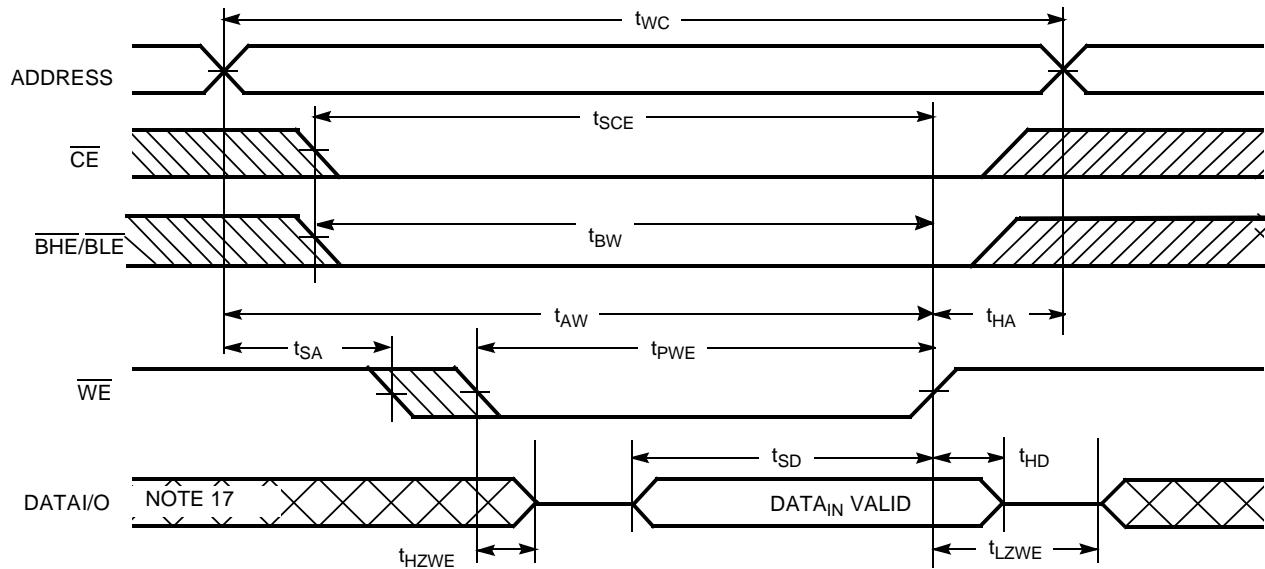
**Write Cycle No. 4 (BHE/BLE Controlled,  $\overline{\text{OE}}$  LOW)**<sup>[16]</sup>
