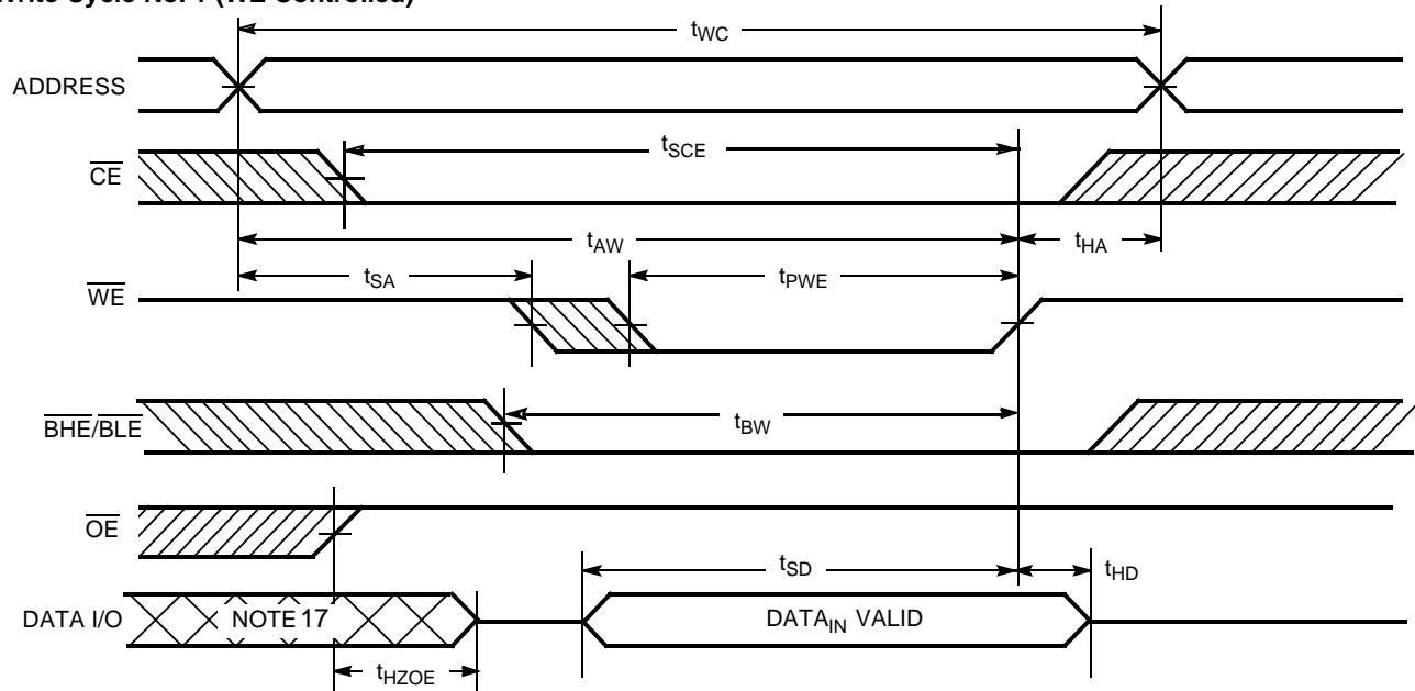
**Write Cycle No. 2 ( $\overline{CE}$  Controlled)** [11, 15, 16]
