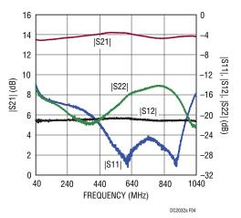
Figure 4. Demo Board DC2032A S-Parameters
