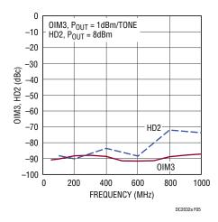
Figure 5. OIM3 and HD2 vs Frequency
