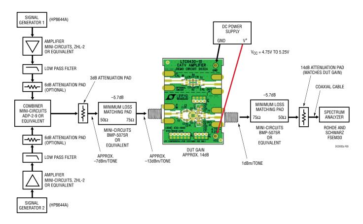
Figure 3. Proper Equipment Setup for IP3 Measurement
