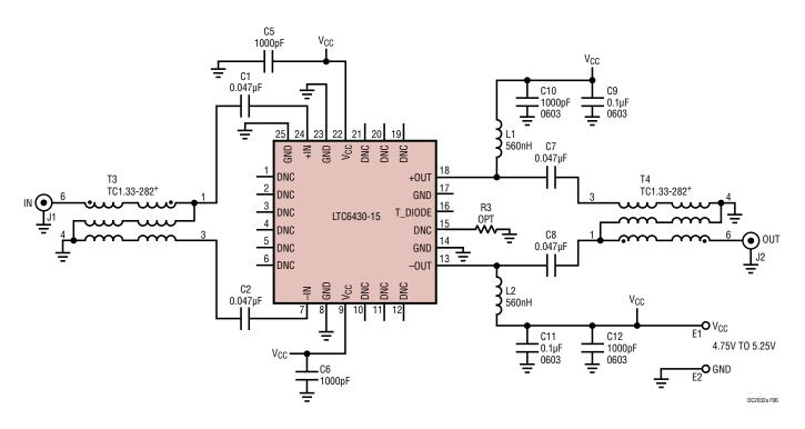
Figure 6. Demo Board DC2032A Simplified Schematic
