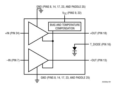
Figure 1. LTC6430-15 Device Block Diagram
