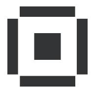
Figure 62. 82583V Solder Mask
