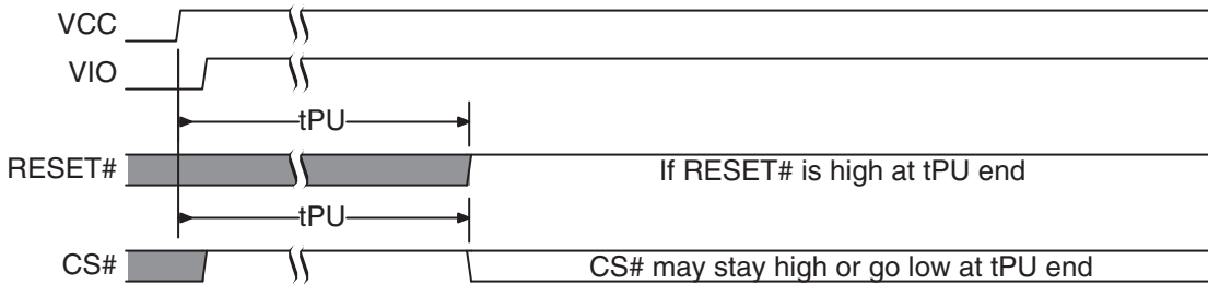
Figure 27. Reset High at the End of POR
