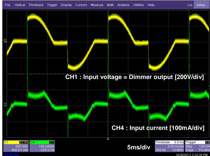
**Figure10.** Dimming operation waveform at
