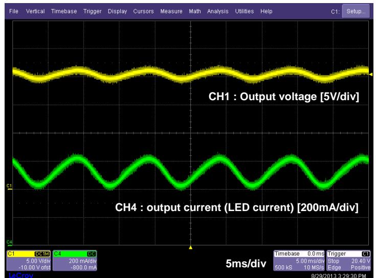
Figure7. Output waveform
