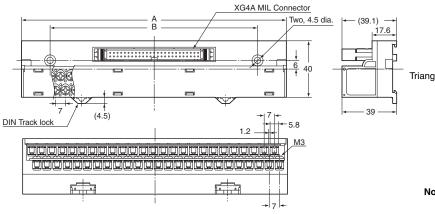
Note: There is only one DIN Track lock located in the center of the terminal block for a 20-pole Unit.
