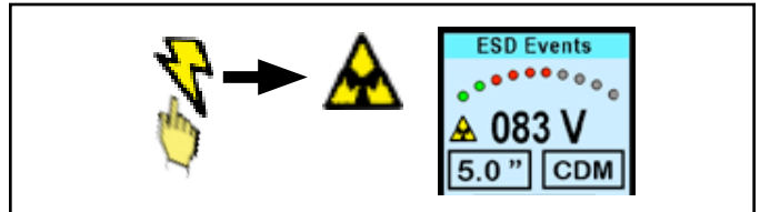
Figure 24. Changing the filter from “True ESD mode” to “All Signal mode”
