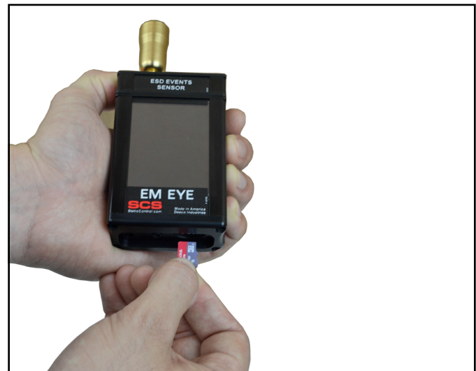
Figure 3. Inserting the SD card into the EM Eye Meter
