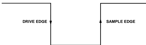
Figure 25. SPI Mode 3 SCLK Edges
