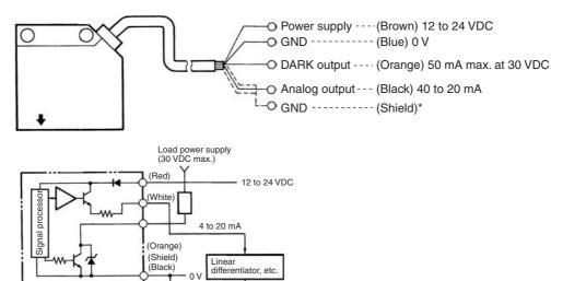
Note: \*The two ground terminals (black and shield) are internally connected. However, the black ground must be used with the red terminal for the power supply and the shield ground must be used with the white terminal for the analog output.
