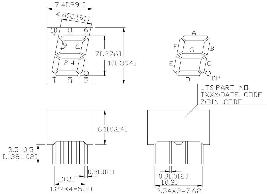
NOTES: All dimensions are in millimeters. Tolerance is ± 0.25 mm (0.01") unless otherwise noted.
