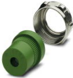
Half screw connection Pg16, made of metal, consisting of rubber seal with one hole and one pressure screw, for type 1 housings, cable [mm] 9 - 13
