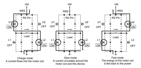
**Output transistor operational function**
