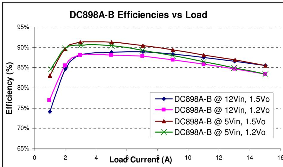
Figure 4. Typical Supply Efficiency vs Load Current of DC898A-B
