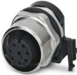
Sensor/actuator flush-type connector, socket, 8-pos., M12 SPEEDCON, A-coded, rear/screw mounting with M12 thread, with polarity protection, with angled solder connection
