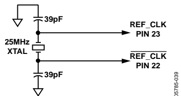
Figure 40. Crystal Configuration for Reference Clock Source
