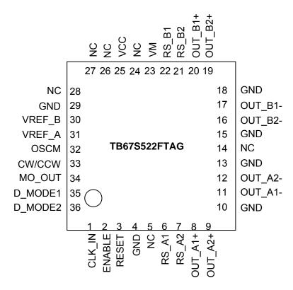
\*: Please mount the four corner pads of the package and the exposed pad to the GND area of the PCB.
