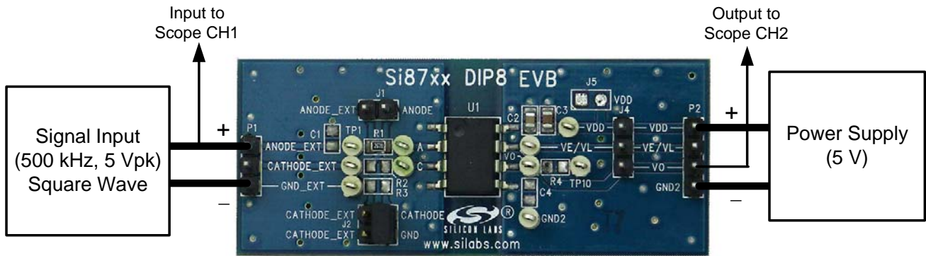
Figure 4. Summary Diagram and Test Setup
