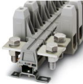
Universal terminal block with mixed connection, cross section: 70 - 240 mm 2 , width: 53 mm, color: gray
